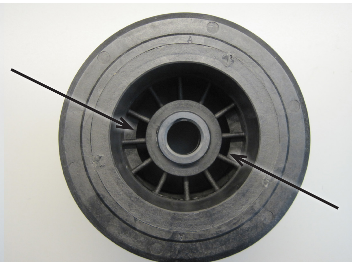
Two Piece Impeller drive hub (no prongs)
