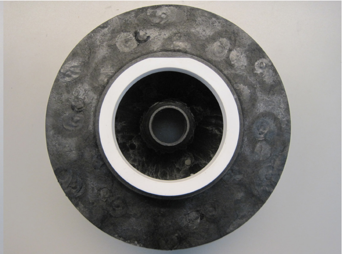
Two Piece Impeller w/ weld pins
