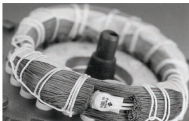
Fig. 18 Thermal switch incorporated in winding
