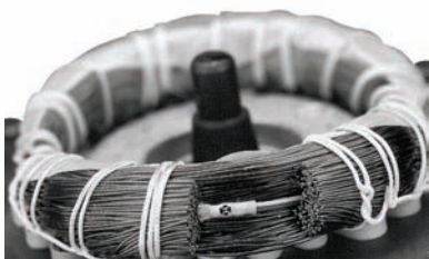
Fig. 16 PTC sensor incorporated in winding
