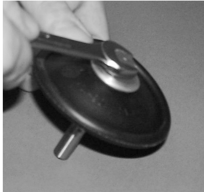
Step 9 Remove shaft and attached outer piston from the center section. Hold the diaphragm and remove outer piston with 7/16" wrench. If unable to remove diaphragm, place shaft in a vise equipped with soft jaws.
