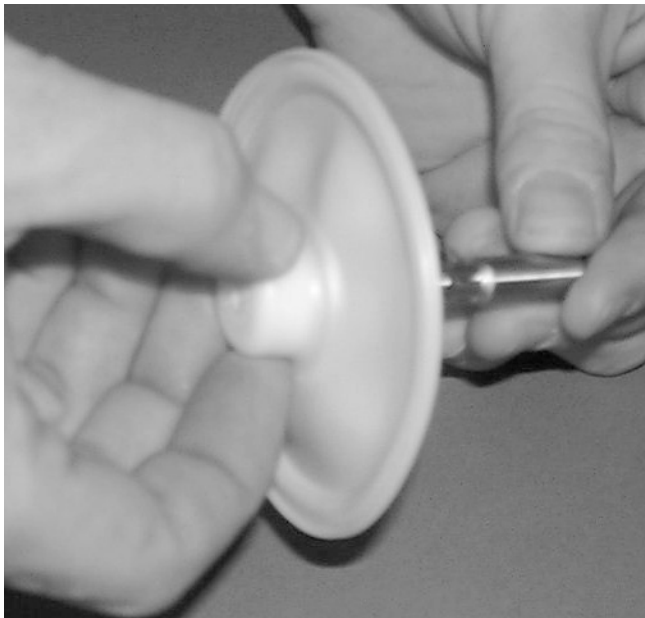
Step 10 For PTFE fitted pumps diaphragms, remove diaphragm by turning in a counter-clockwise direction.
