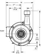
Maximum Solids Handling Capacity: 1/8" Diameter
