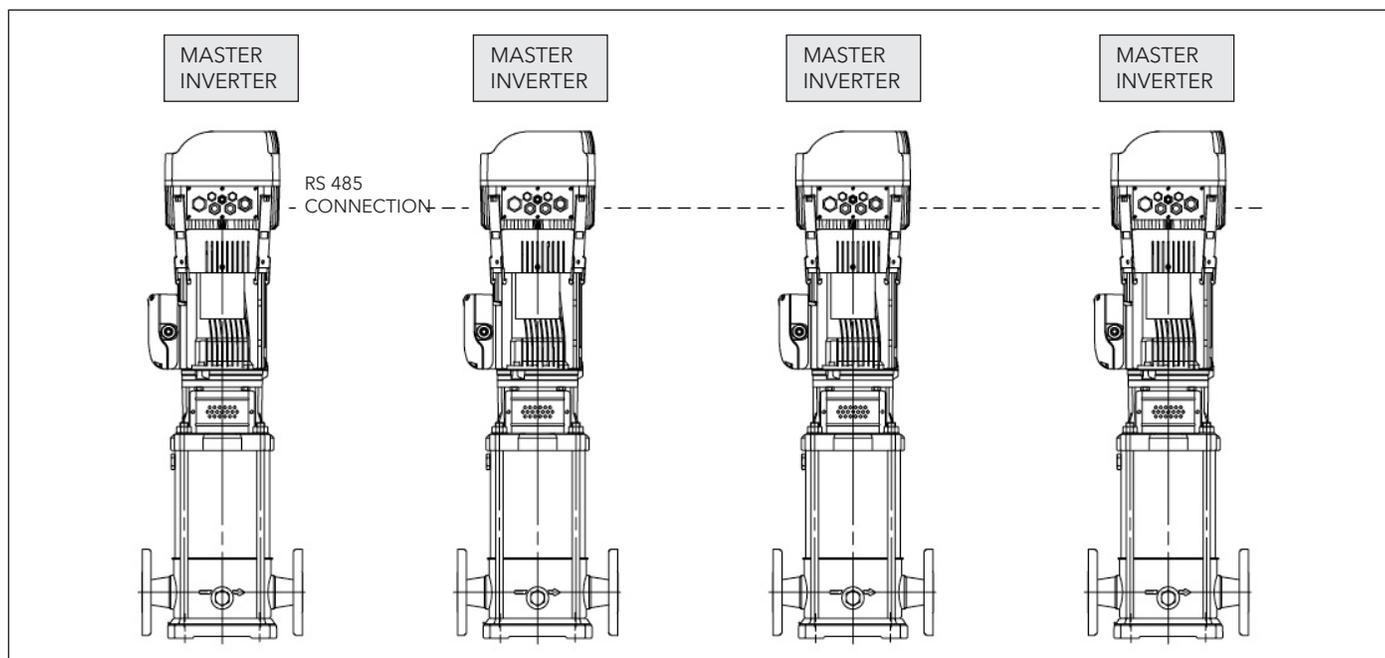
With the "master" version of the Hydrovar, it is possible to connect up to 8 Hydrovar controller pumps together in parallel. Complete lead/lag and auto alternation.
