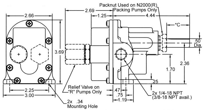
\*C Dim: 1.03 for Packing Pumps, 1.81 for S3 & S5 Lip Seals, 1.51 for S16 & S17 Mech. Seals
