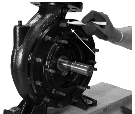
20. Remove pump cover and the impeller.
