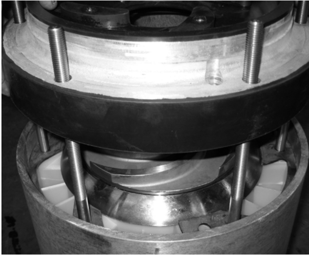
Pic #2 High head upper diffuser installation
