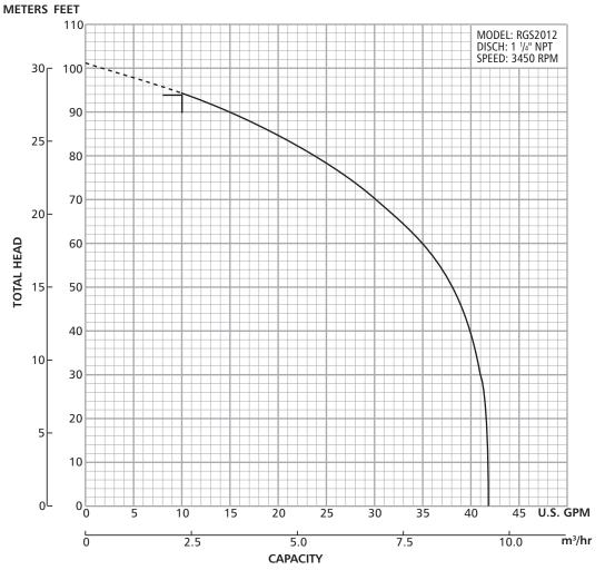
$\Box = A \frac{1}{4}$  minimum discharge pipe requires a minimum flow of 10 gpm to maintain a 2 ft./sec. scouring velocity. Flows less than 10 gpm will allow solids to settle in the pipe.
