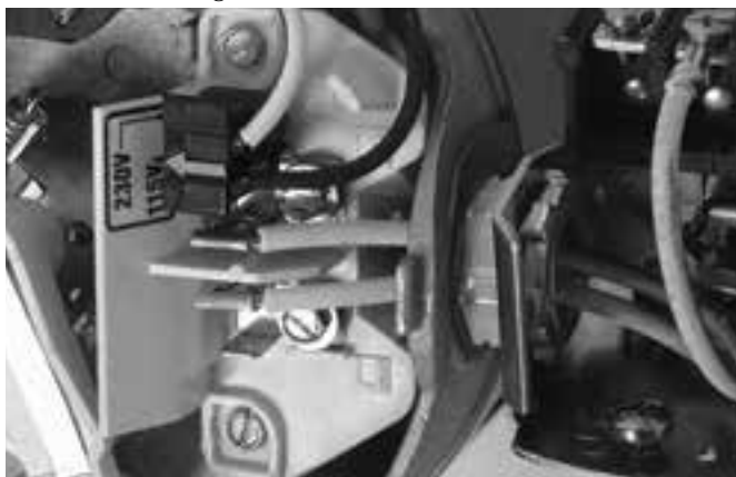
Figure 9: Voltage set to 115 V, Plug Type
