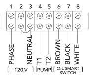
\* For 240V, remove jumper and supply power to terminals 1 and 2, with neutral on 3.
