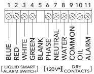
\* Hook up separate 120V supply here or jump from pump terminal 1 and 3 to alarm terminal 6 and 7 for power.
