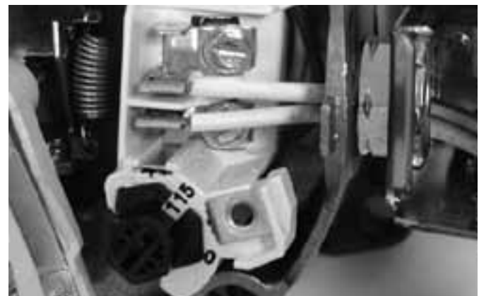
Figure 11: Voltage set to 115 volts, Dial Type
