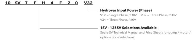
HV - Hydrovar Variable Speed Drive
