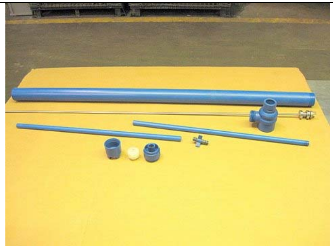
Picture illustrates pump completely disassembled.
