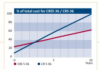
This curve shows the typical impact of energy savings provided by the CRE pumps in water supply and boosting applications. Compared to a standard CR, the CRE begins to yield profits after just 2.5 years – and continues to do so for years thereafter.
