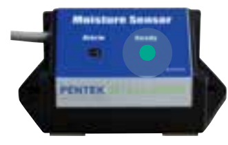
Fig. 3 Green "Ready" Indicator Illuminated
