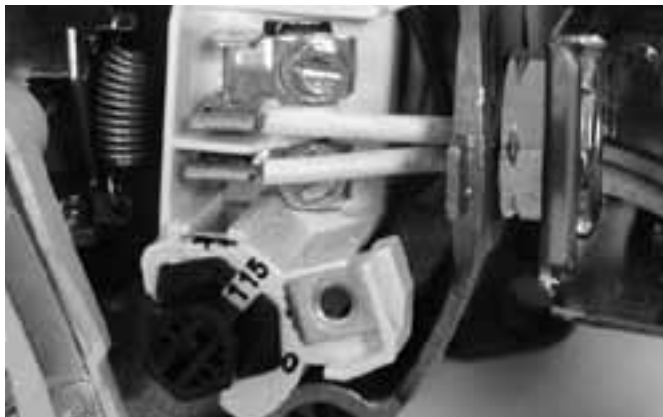
Figure 7: Voltage set to 115 volts, Dial Type
