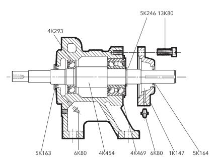
L-Group power frame for models 3756 mechanical seal and packed box pumps
