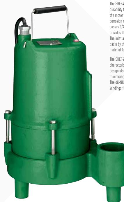
The HYDROMATIC<sup>®</sup> SHEF45 submersible pump is specifically designed to meet the demands of residential septic tank effluent or sump applications. The 2 inch NPT discharge pump features an energy-efficient 1/2 horsepower motor, manual version. The SHEF45 can handle capacities up to 87 gallons per minute and heads to 44 feet.
