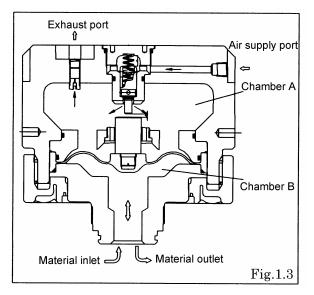
When the pressure of chamber B is increased by pulsation caused by pump operation, the diaphragms go up to increase the capacity of chamber B, so that the pressure is absorbed. When the pressure of chamber B is reduced, the diaphragms are caused to go down by the pressure of chamber A to reduce the capacity of chamber B, so that the pressure is increased. This operation acts as an air cushion to absorb the pulsation of liquid.
