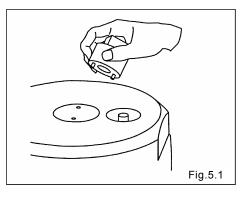
Use the dedicated tool 1, a socket for a guide (option 804131) and a 24-mm wrench to remove the spring sheet.
