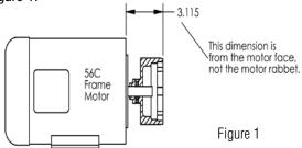
Align set screw (item 6B) with flat or key slot on the motor shaft and tighten both setscrews with a 5/32" Allen wrench to 70 in.-lbs. (7.9 N-m).
