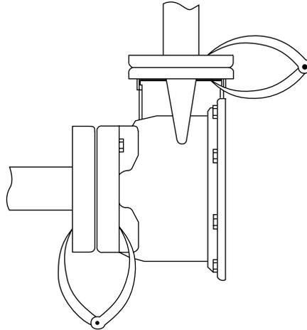
1. Check the tightness of all hold-down bolts before checking the alignment.
