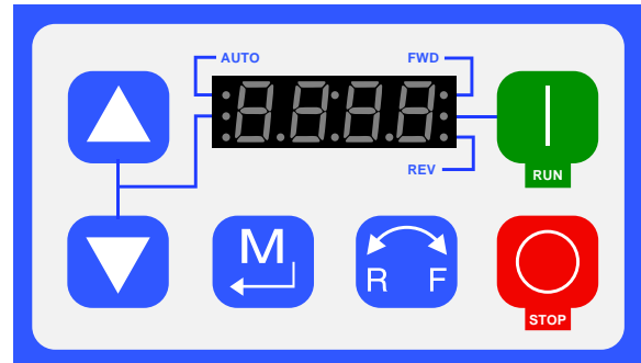
Figure 11 VFD Control Panel
