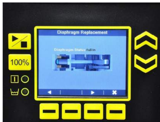
Figure 31: Diaphragm Replacement (Full In)
