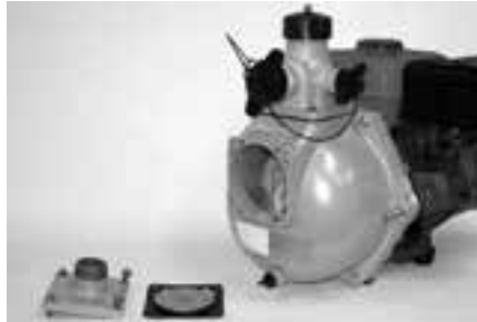
Figure 29: Remove Flap Valve
