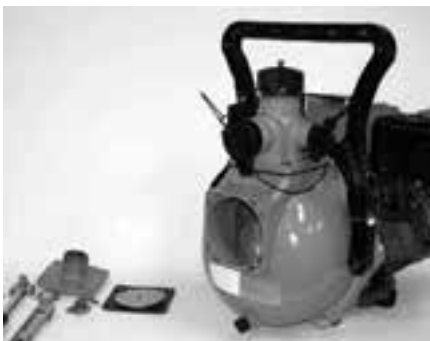
Figure 2: Suction Flange Removal
