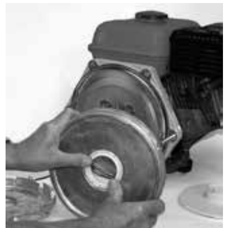
Figure 39: Remove Wear Ring
