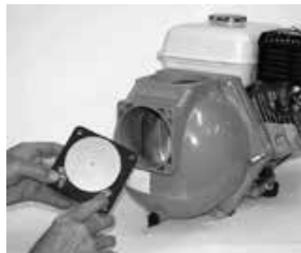
Figure 24: Install Flap Valve
