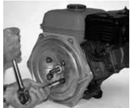
Figure 12: Seal plate Removal
