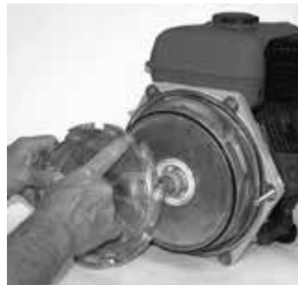
Figure 52: Install Front Diffuser
