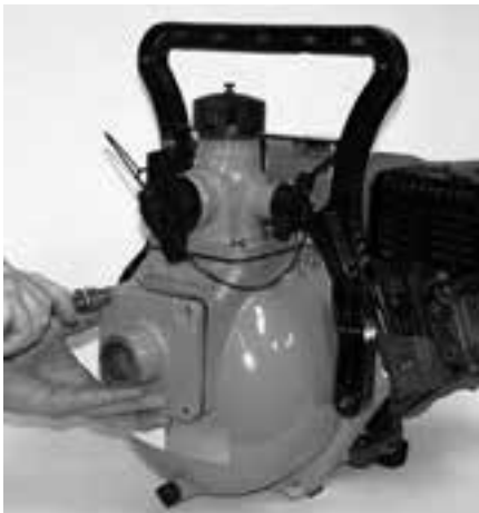
Figure 1: Suction Flange Removal
