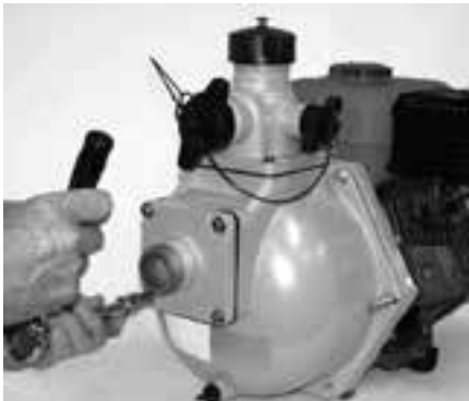
Figure 28: Remove Suction Flange
