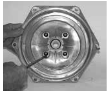
Figure 13: Remove Bolt Seals
