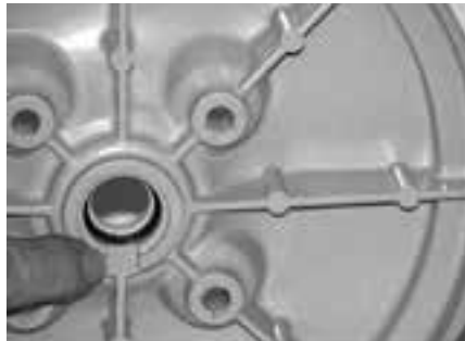
Figure 45: Seal Plate Drain Location
