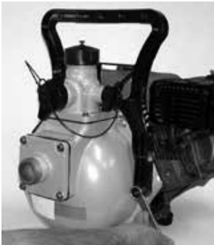
Figure 27: Remove The Handle
