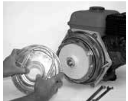
Figure 33: Remove Wear Ring
