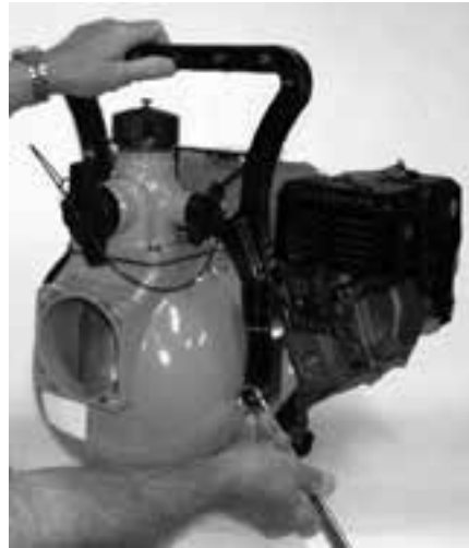
Figure 3: Remove Front Bolts
