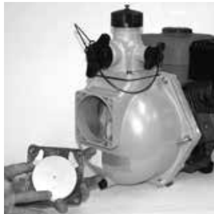
Figure 58: Install Flap Valve
