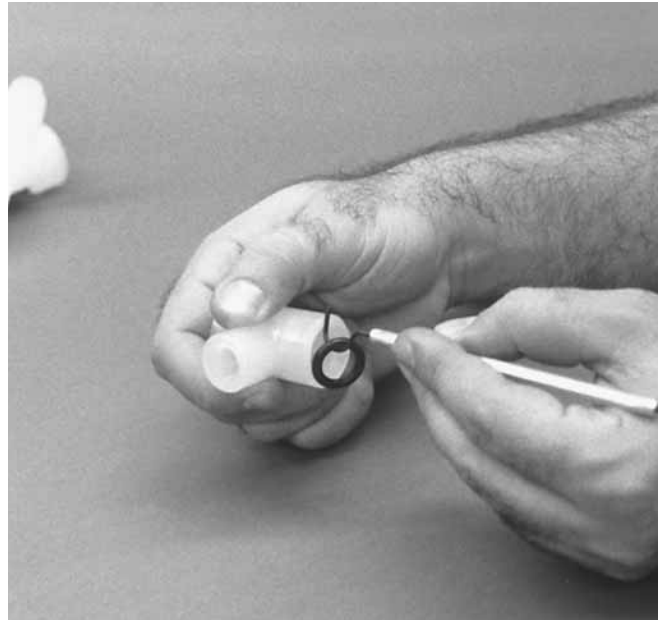
Step 9 Carefully remove tee-section o-ring. Inspect o-ring for wear and replace with genuine Wilden parts if necessary.
