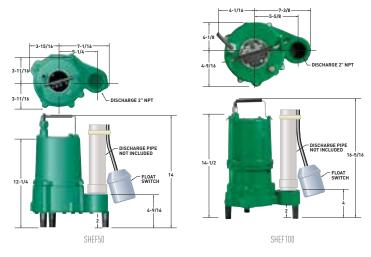
All dimensions in inches. Metric for international use. Component dimensions may vary ± 1/8 inch. Dimensional data not for construction purpose unless certified. Dimensions and weights are approximate. On/Off level adjustable.
