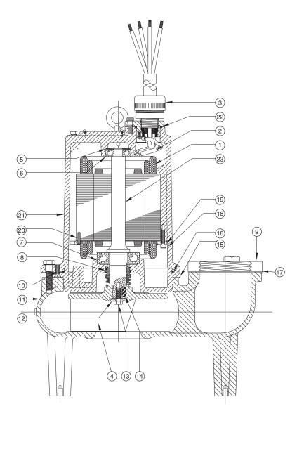
Notes: S — Parts in Seal Kit C — Parts in Carbide Seal Kit — Fill Oil to above Motor Windings
