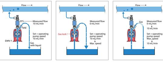
The auto air vent valve bleeds gas and liquid out of the pump chamber. However, pump output is maintained due to the feedback control from the flow sensor.
