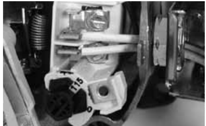
Figure 7: Voltage set to 115 volts, Dial Type
