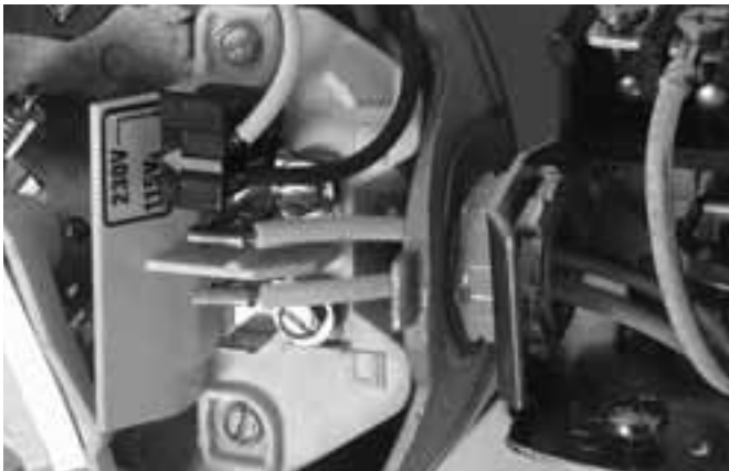
Figure 5: Voltage set to 115 volts, Plug Type
