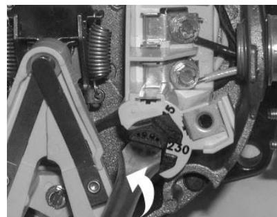
Figure 3: Changing the Voltage Setting
