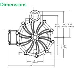
Also available 2" x 2" or 3" x 2" 150 lb. ANSI/ISO PN20/PN40/ JIS 10K or 63mm x 63mm union connection. Flanges are in compliance with bolting dimensions only.
