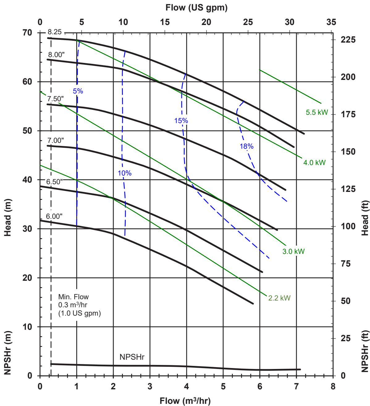
Impeller trims are available in 1/8" diameter increments (ex: 4.13", 6.13") between all curves.
