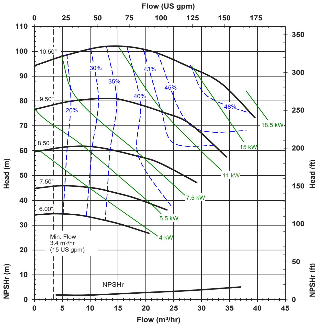
Impeller trims are available in 1/8" diameter increments (ex: 4.13", 6.13") between all curves.
