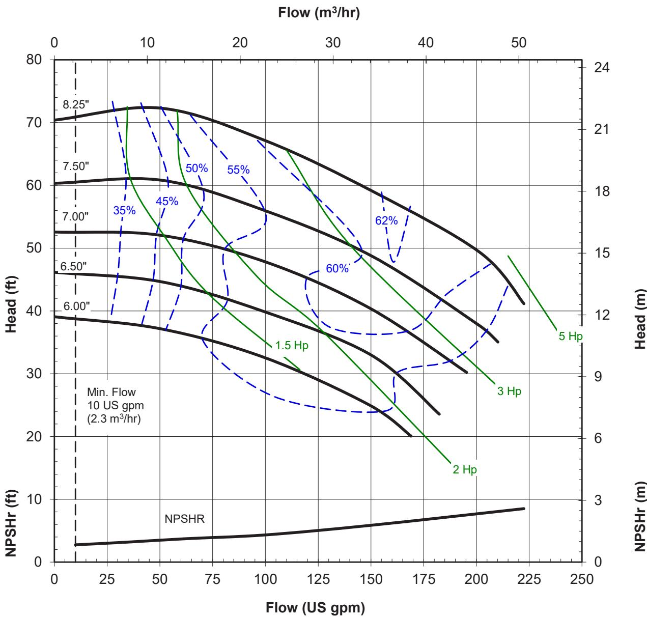
Impeller trims are available in 1/8" diameter increments (ex: 4.13", 6.13") between all curves.
