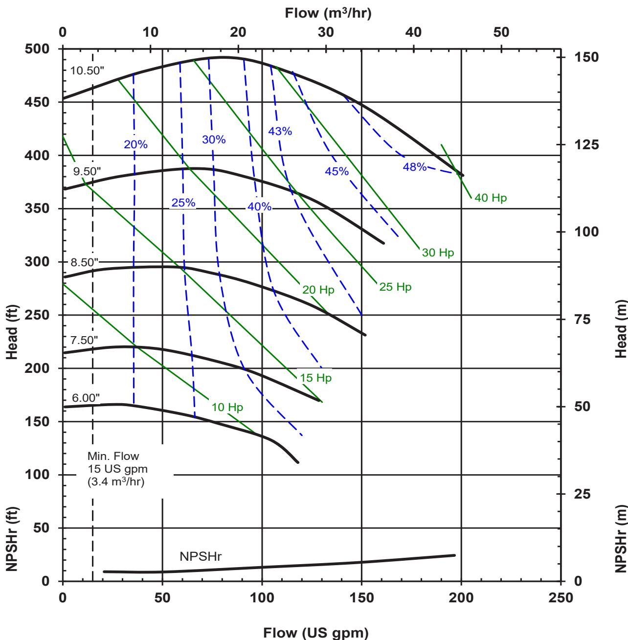
Impeller trims are available in 1/8" diameter increments (ex: 4.13", 6.13") between all curves.
