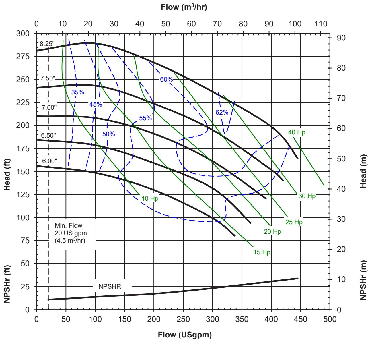
Impeller trims are available in 1/8" diameter increments (ex: 4.13", 6.13") between all curves.
